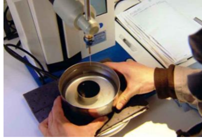
Fig. (1): Penetration test.
