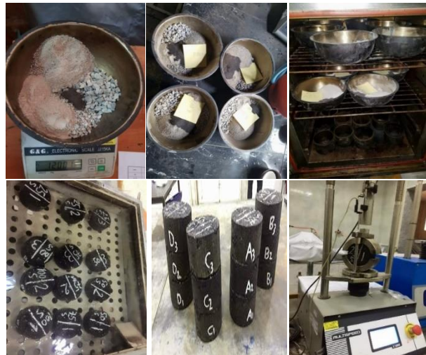
Fig. (4): Marshall Test preparation specimens with IWP.
