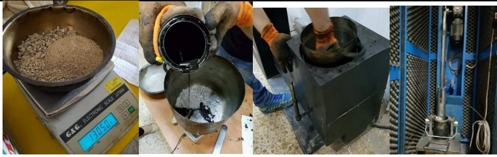
Fig. (2): Prepare Marshall specimens to determine OAC.
