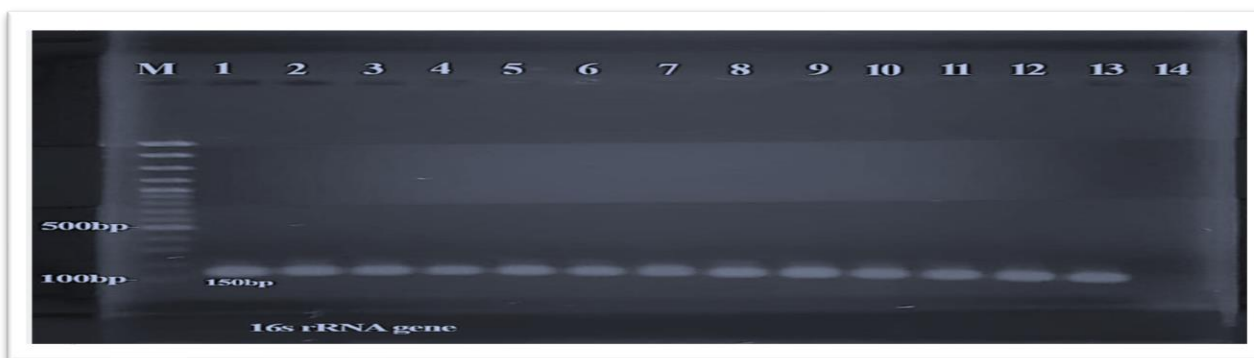
Fig. (2): Bands of PCR product for 16 S rRNA of A. baumannii on 1 % agarose gel. Lane M is DNA ladder (1500-100bp).
