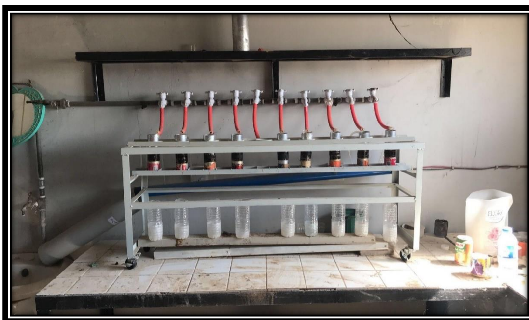
Fig. (2.13): a picture showing the apparatus used for measuring Saturated hydraulic conductivity (HC).
