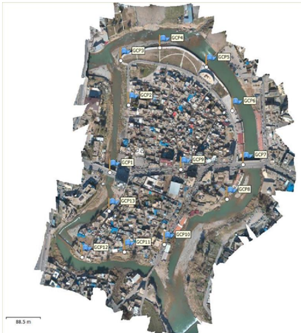
Fig.(2): -Location of 13 GCPs and 2 check points Marking
