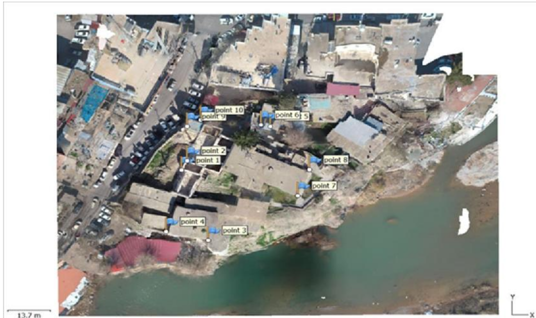
Fig.( 8): -10 Checkpoints for Qishla Building
