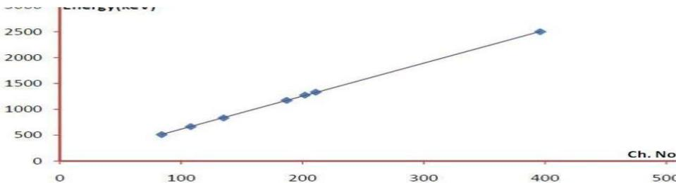
**Fig. (3):** Calibration curve of channel-energy of NaI (Tl) detector.
