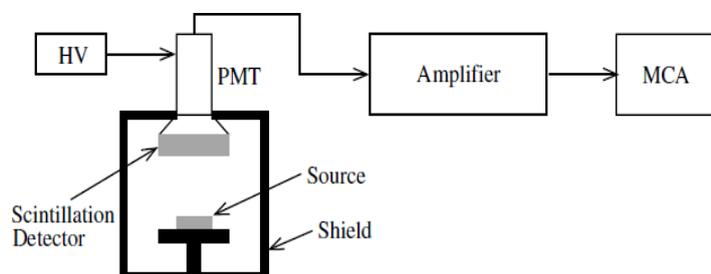
**Fig. (2):** A spectrometer system is depicted as a block diagram [23]
