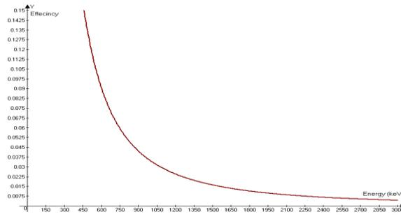
Fig. (4): The efficiency calibration curve of NaI (TI) detector
