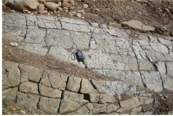
**Fig. (4):** Fractured (marl limestone) of the Shiransh fm. at siktan dam site.
