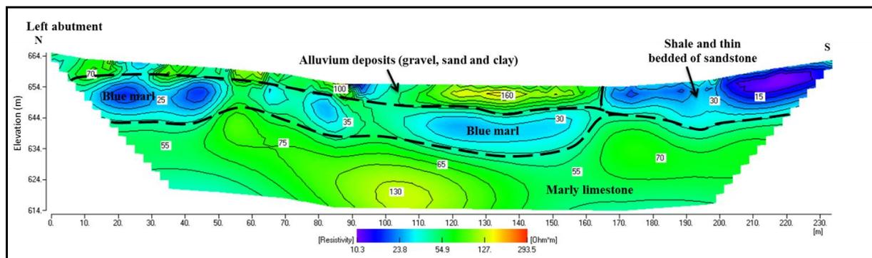
Fig. (9): Inverse resistivity model along profile 1 which is parallel to the proposed dam axis.
