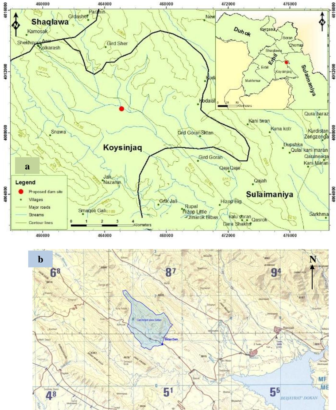
**Fig. (1):** a- Location map of the Proposed Dam. b- Siktan dam topography, catchment areas and reservoir (GDDR, Geotechnical Internal Report, 2014).
