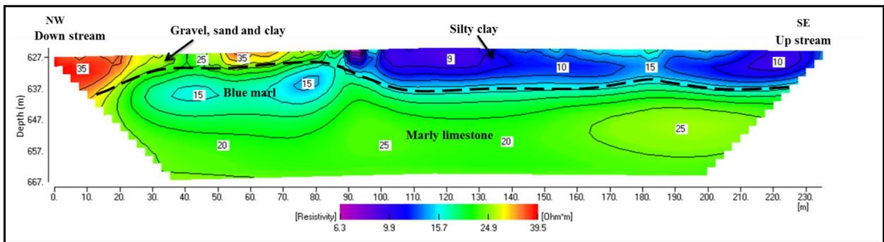
Fig. (11): Inverse resistivity model along profile 3.
