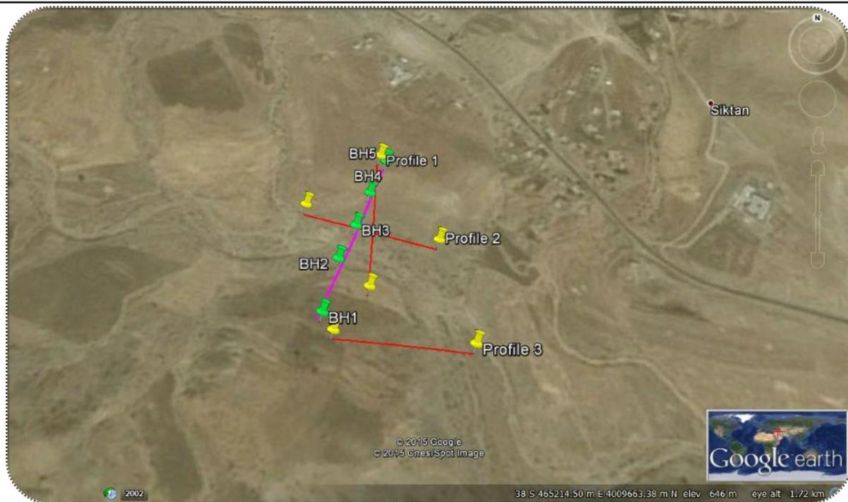
**Fig. (8):** Satellite Image showing the 2D electrical resistivity profiles and location of the boreholes at Siktan proposed dam.
