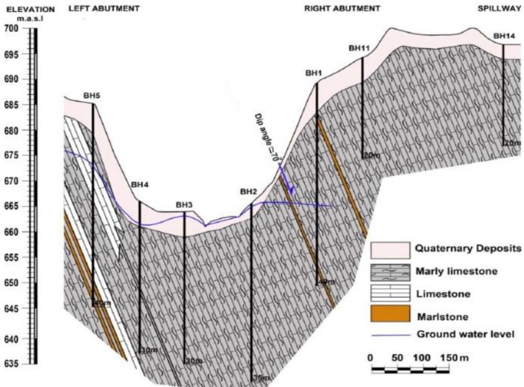
Fig. (12): Geological cross section along Dam axis (GDDR, Geotechnical Internal Report, 2014).
