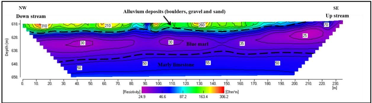
Fig. (10): Inverse resistivity model along profile 2 which is perpendicular to the proposed dam axis.
