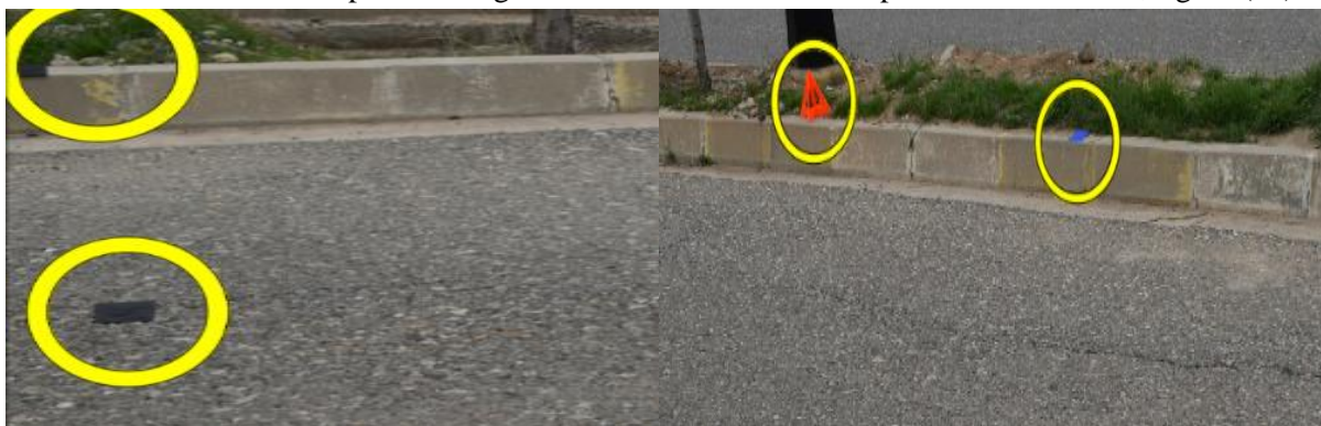
Fig. (13): GCP (black and blue sticker) with the origin point (warning triangle)
