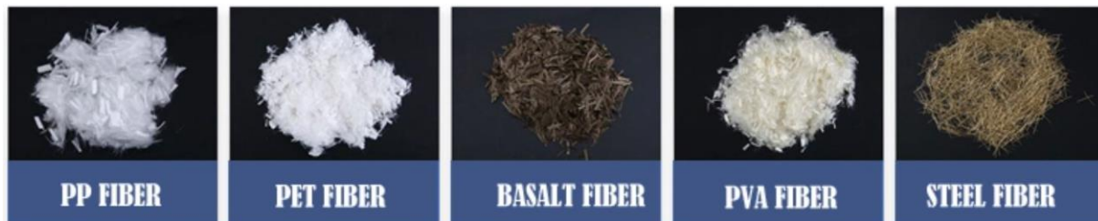
Fig. (3): Different types of fibers are used in roller compacted concrete pavement
