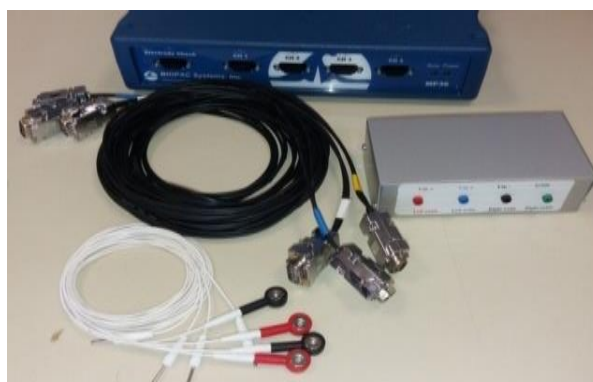
Fig.(6):- Designing Electrodes and wires to connect Biopac System with box and Subject.
