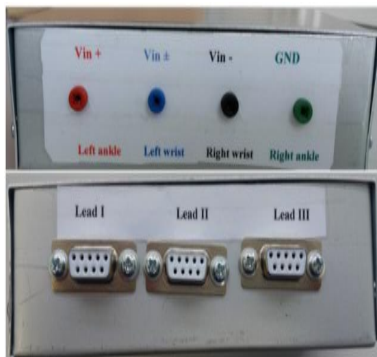
Fig.(5):- Physical design of 4 electrodes to connect with Biopac System.
