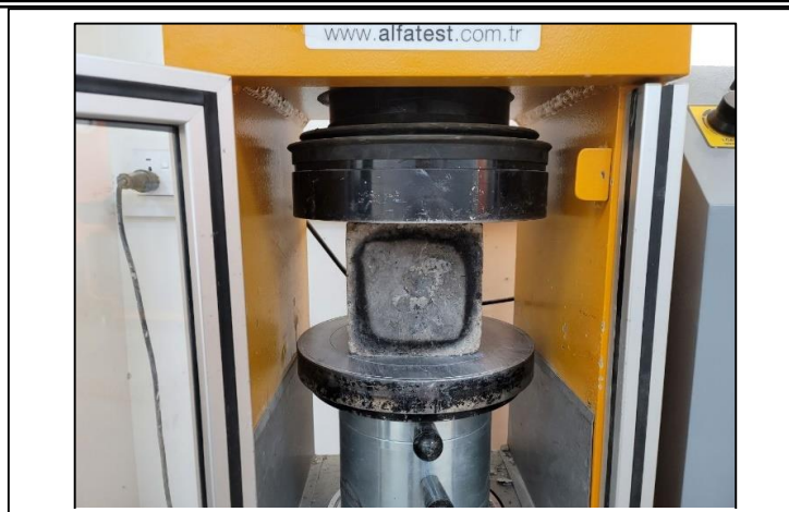
Fig.( 4):- Sample from mix HSGC-4 after being subjected to 1000 °C
