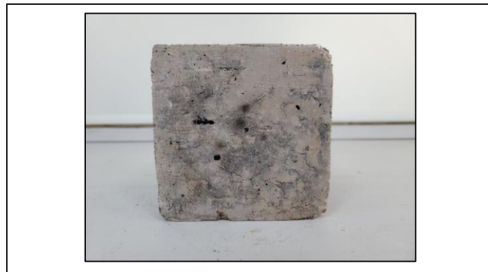
Fig.( 6):- Cracks on the surface of the sample after being subjected to 500 °C
