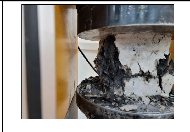
Fig.(7):- Chemical composition change of mix HSGC-4 after exposure to 1000 °C
