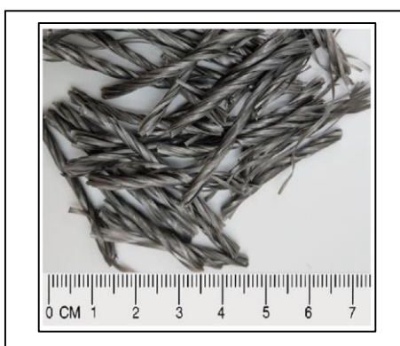
Fig.( 3):- Physical appearance of the PP fibres.
