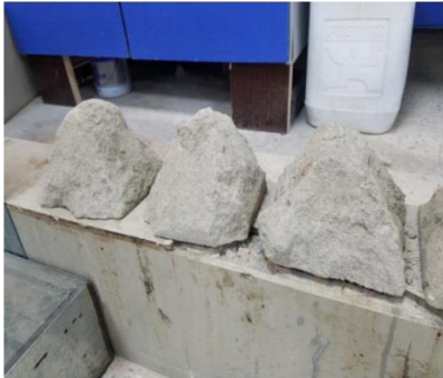
Fig.(6):-Collapse form of M(0)
