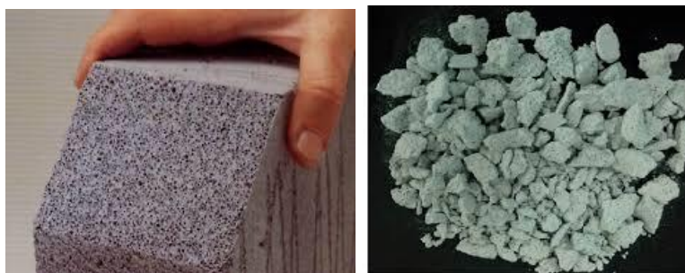
Fig.(5):- Autoclaved Aerated Concrete produced from lightweight aggregate
