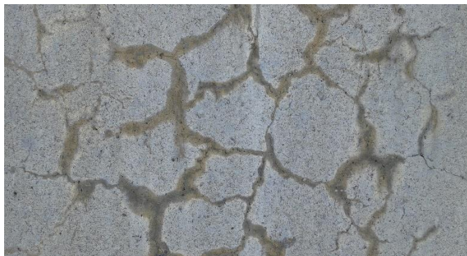
Fig.( 8):- Alkali-aggregate reaction [1]
