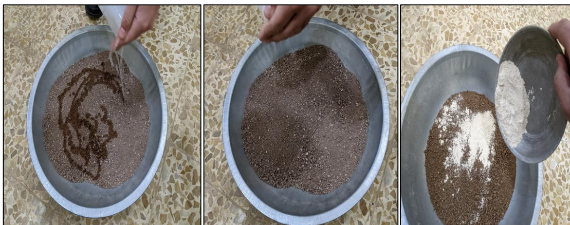
Fig.(3): -Mixing the stabilizers with soil
