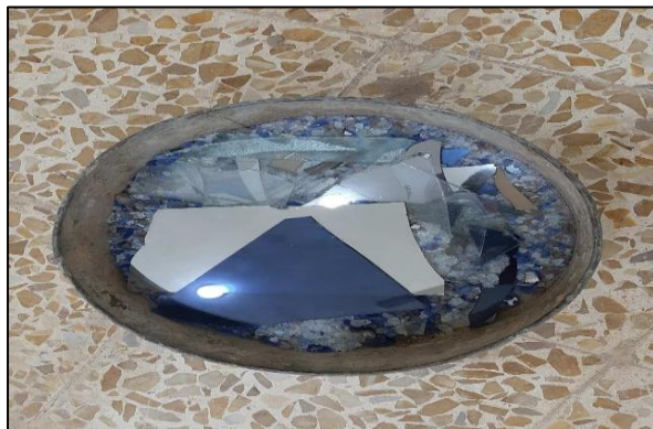
a: Glass Waste used for tests before pulverization
