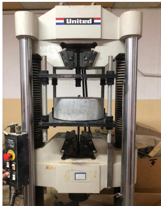
Fig.( 4 ):- Pull-Out Test Setup
