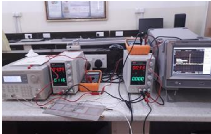
Fig. (20):- Practical test setup of the RF amplifier circuit.
