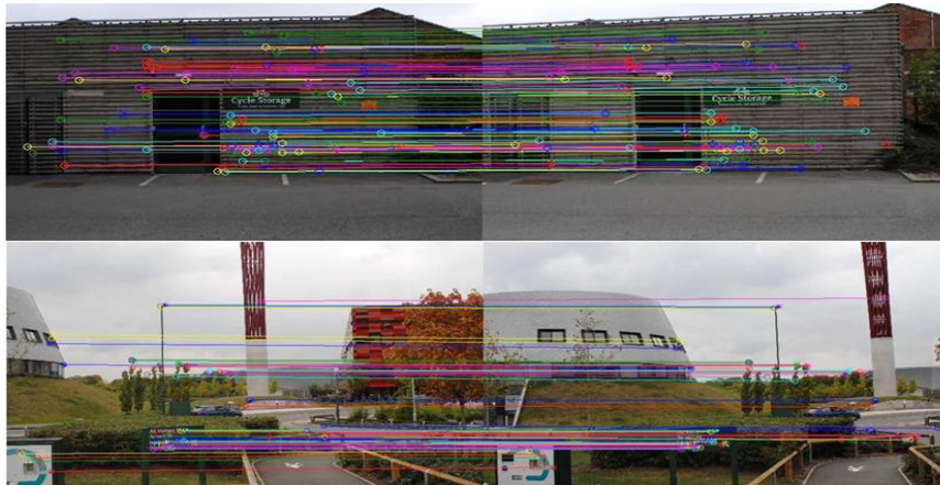
Fig. (3): Examples of automatic image matching using SIFT (Up) and SURF (Down)
