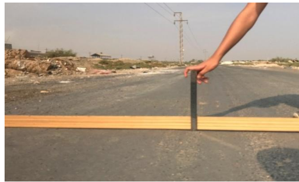
Fig. (6) : Rut depth measurements on test road
