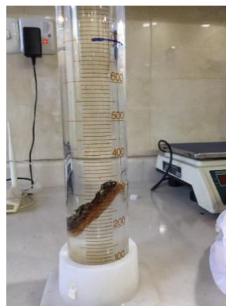
Figure 2.2 Measuring of wet volume (Archimedean principle)
