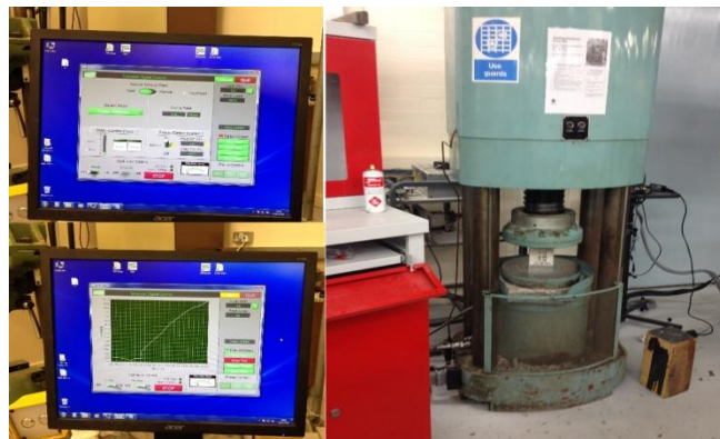
Fig. (5): Automated computerised compressive test
