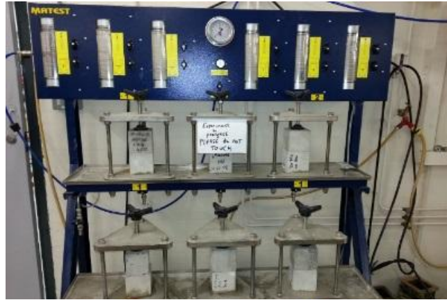
Fig. (3): Permeability testing device
