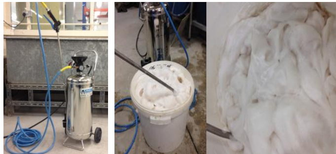
Fig. (1): The device used to generate the foam
