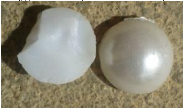
Fig. (9): Difference between plastic pearl material roughness and its surface roughness
