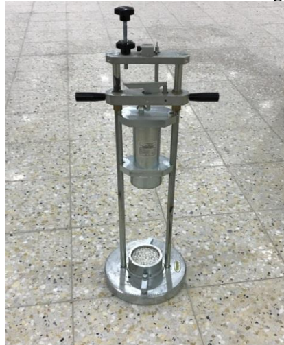
Fig.(2): Impact value test for plastic pearls
