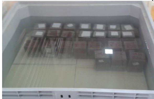
Fig. (3): Concrete cubes curing
