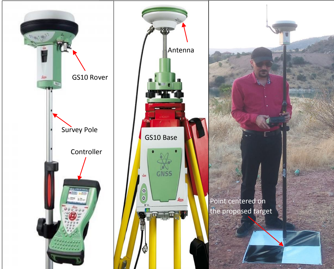
Fig. (6): Leica Viva GS10, base and Leica viva GS15, rover.
