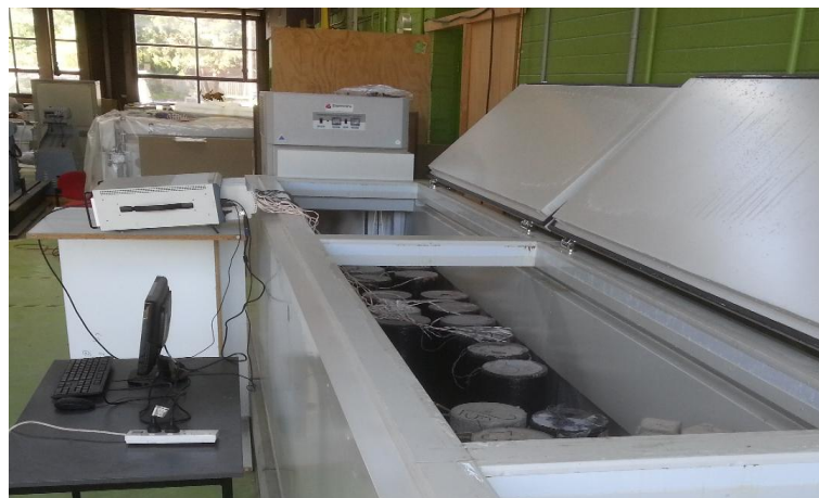
Fig. (1): Monitoring strain in concrete and steel during storage of columns.
