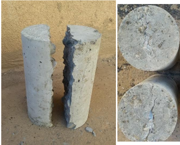
Fig.(6): Sample after splitting tensile test
