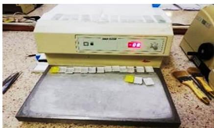
Fig.(4): LEICA EG 1130 to pre-cool the paraffin embedded biological specimen at -30C°
