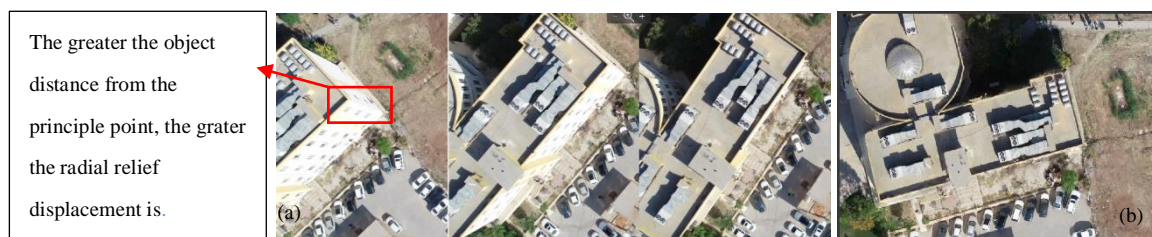
Fig. (12. a): Relief displacements on high building, b) Orthophotos without relief displacement
