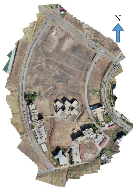
Fig. (9): Orthomosaic, colour 3 bands, uint8 with coordinates system WGS 84 / UTM zone 38N
