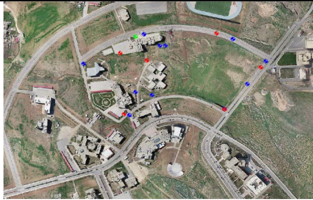
Fig. (1): Area of study overlain GCPs represent in red color and check points represent in blue color
