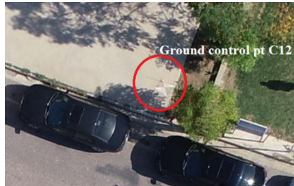
Fig. (6): A sample of GCPs appear in the image taken by UAV at 80m altitude.
