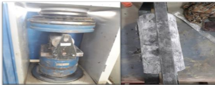
Fig. (4): Specimens for splitting tensile strength evaluation
