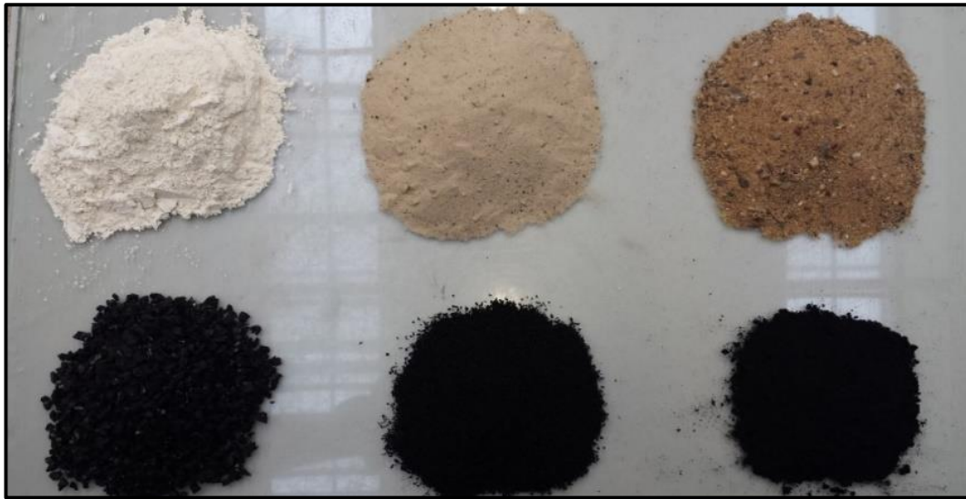
Fig. (1): Top: China clay (left), Levenseat sand (middle), concrete sand (right). Bottom: shredded tyre 2–6 mm (left), 12 mesh (middle), 50 mesh (right)
