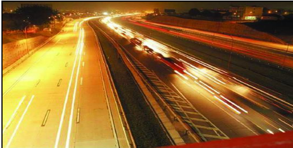
Fig. (4): Visibility at night between concrete road (Left) and asphalt road (Right) (ACPA, 2007)
