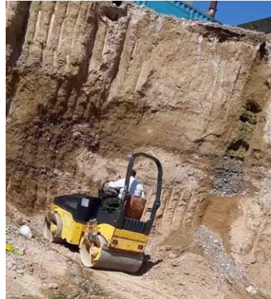
Fig. (7) :The heavy machine that used as seismic source vibrator at tower-building site
