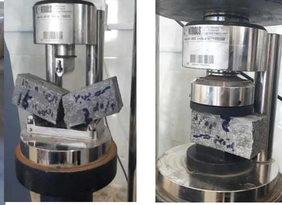
Fig. (5): Samples under flexural and compression machines apparatus
