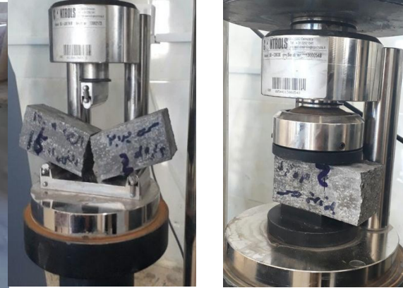
Fig. (5): Samples under flexural and compression machines apparatus
