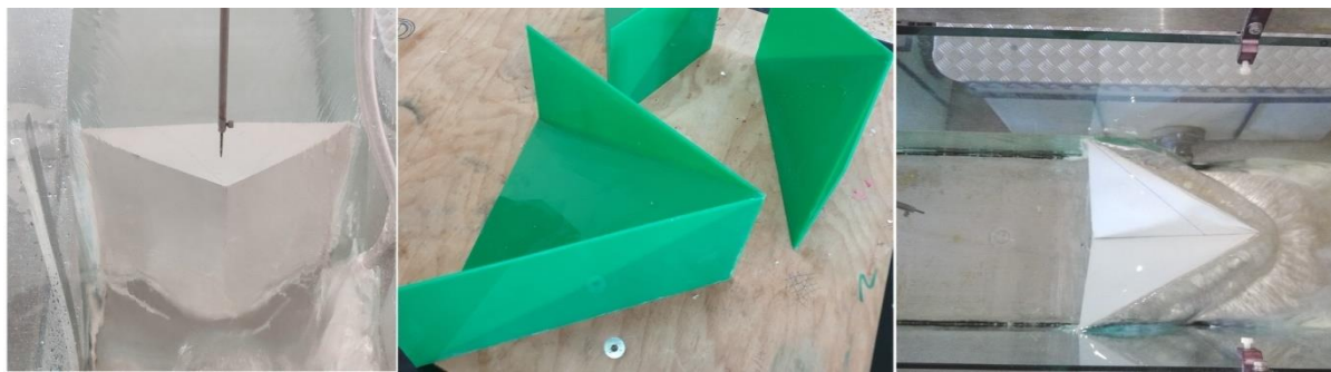
(a) Triangular plan form flat top weir (b) Triangular plan form piano weir (c) Triangular plan form semi piano weir
