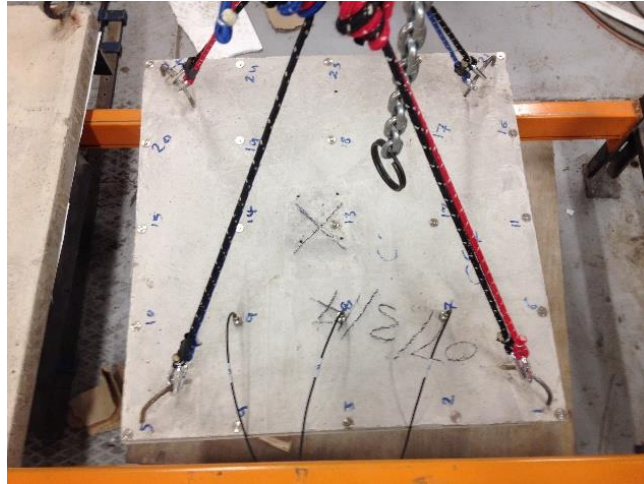
Fig. (2): Vibration grid measurement points.
