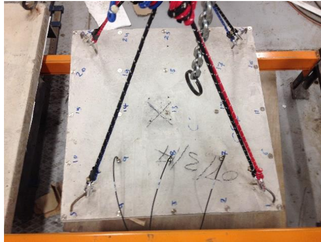
Fig. (2): Vibration grid measurement points.
