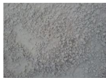
Fig. (2): Thermostone aggregate
