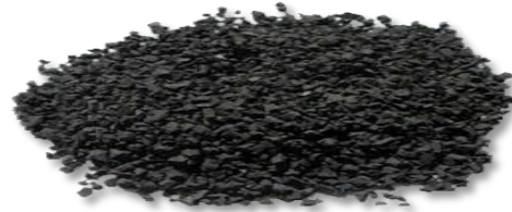
Fig. (4): Rubber from waste tires used
