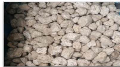
Fig. (1): Lightweight claystone coarse aggregate
