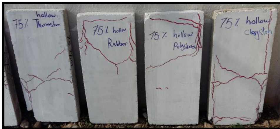
C - Hollow slabs at the replacement ratio of 75%
