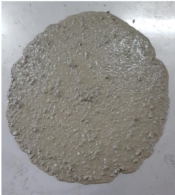
Fig. (5.1): Flow test of mix SCC(M60)
